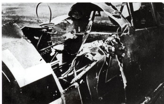
'Black 12', the Bf 109 G-6 of Lt. Heinicke from 10./JG 5 after a forced landing at Petsamo on 17 October 1944. The aircraft was hit in the fuselage spine by a large calibre cannon, possibly a 37 mm round from an Airacobra, but still managed to reach the airfield and make a wheels-up emergency landing, whereupon the Messerschmitt broke its back. The aircraft has the tall tail fin and standard RLM 74/75/76 scheme with comparatively heavy mottling in the two greys. The spinner seems to have a very broad white spiral. Note that the older type of canopy is fitted, having been ejected next to the aircraft. Numbers and Gruppe disc are black with a thin white outline. The absence of any visible theatre markings is noteworthy (Coll. Brekken).
