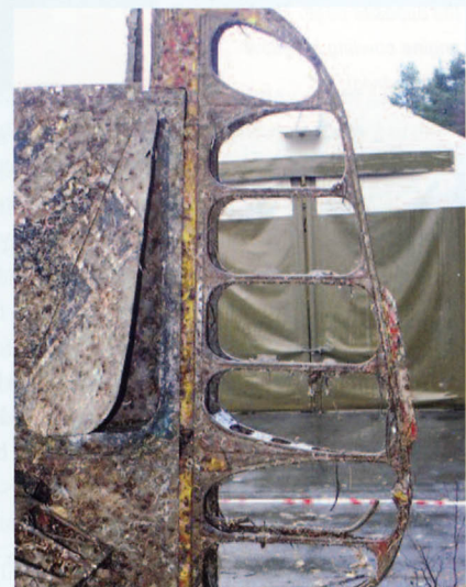
Top and below: Further detail views showing the unmodified early type exhaust slots and the rudder framing devoid of fabric but still showing traces of yellow paint and the port inner cannon bay (Coll. Dybvig).
