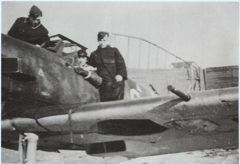
Several of the features of a converted E-1 can be seen in this photograph. The circular patch on the wing leading edge just inboard of the retro-fitted MG FF M covers the aperture for the MG 17. This Emil was therefore probably built as an E-1 and has also received a new canopy and the external armoured wind shield. Of interest is the canvas cover tied around the wing root to prevent excessive wear. This aircraft was 'White 8' of either 4. or 7./JG 5 (Coll. Brekken).
