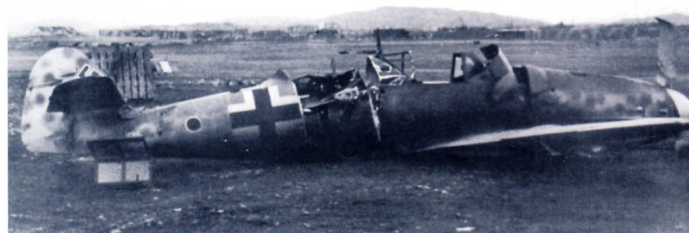
'Black 12', the Bf 109 G-6 of Lt. Heinicke from 10./JG 5 after a forced landing at Petsamo on 17 October 1944. The aircraft was hit in the fuselage spine by a large calibre cannon, possibly a 37 mm round from an Airacobra, but still managed to reach the airfield and make a wheels-up emergency landing, whereupon the Messerschmitt broke its back. The aircraft has the tall tail fin and standard RLM 74/75/76 scheme with comparatively heavy mottling in the two greys. The spinner seems to have a very broad white spiral. Note that the older type of canopy is fitted, having been ejected next to the aircraft. Numbers and Gruppe disc are black with a thin white outline. The absence of any visible theatre markings is noteworthy (Coll. Brekken).
