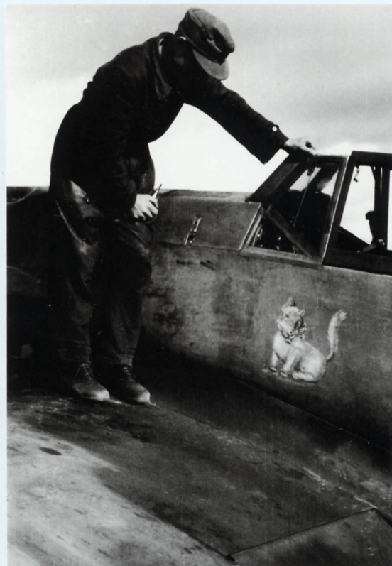
A detail view of the port wing root. There are three colours on the wings, a very light shade around the wing cross (to left), a very dark colour in the centre (RLM 70) and a lighter between these, probably RLM 79, 70 and 75 respectively. Note the very weathered state of the aircraft at the time the picture was taken (Coll. Horst Kube).
