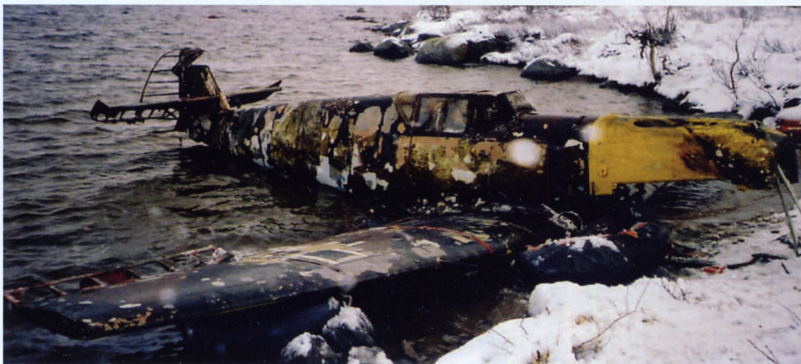
Several of the features of a converted E-1 can be seen in this photograph. The circular patch on the wing leading edge just inboard of the retro-fitted MG FF M covers the aperture for the MG 17. This Emil was therefore probably built as an E-1 and has also received a new canopy and the external armoured wind shield. Of interest is the canvas cover tied around the wing root to prevent excessive wear. This aircraft was 'White 8' of either 4. or 7./JG 5 (Coll. Brekken).
