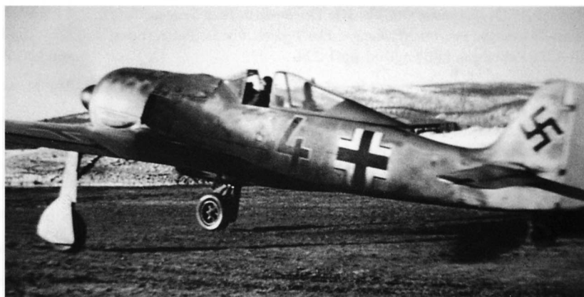
Fw 190 A-3, 'Black 4', seen just after landing with an empty bomb rack. The camouflage comprises the standard greys, while the rudder is yellow (Coll. Horst Kube).
