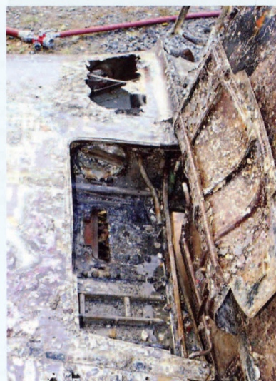
Top and below: Further detail views showing the unmodified early type exhaust slots and the rudder framing devoid of fabric but still showing traces of yellow paint and the port inner cannon bay (Coll. Dybvig).
