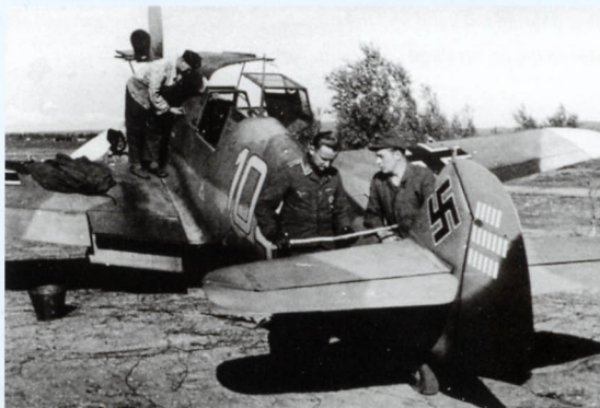
Above: Two views of 'Yellow 10' after having received some repainting (possible after sustaining combat damage) around the fuselage below the numeral. This was applied with a darker colour which may have been RLM 02. Note that the circular compass hatch has also been replaced and the missing part of the numeral has not been repainted. These views also indicate that what appears to be a fourth colour around the fuselage cross on the spine is probably a rather thinly sprayed RLM 70. The photograph above shows part of the upper surface pattern in three colours RLM 79/75/70) and the white wing tips (Coll. Döbrich).
