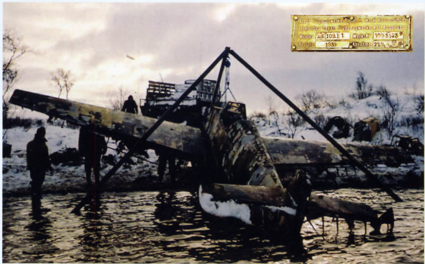
W.Nr. 3523 during the salvage process. Here substantial remains of paint can be seen, although much of the RLM 74 and 75 on the fuselage has peeled off, revealing the RLM 79 Sandgelb underneath (Via Mark Sheppard).
