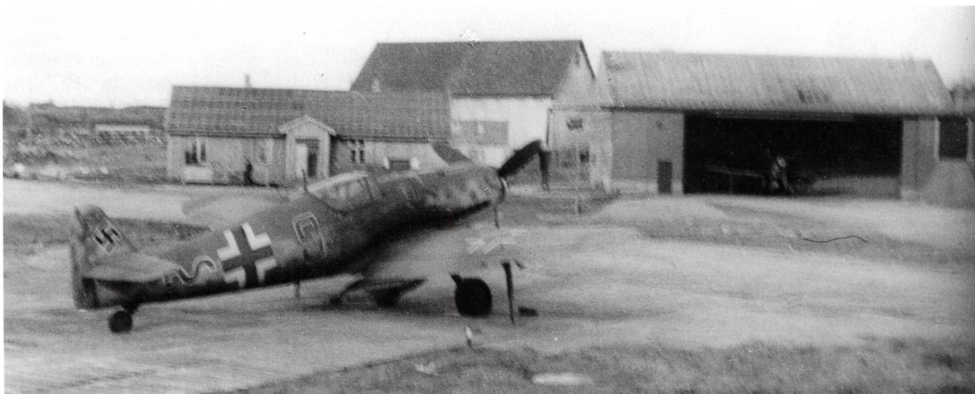
Bf 109 G-14, 'Blue 9' from 16./JG 6 flown by Fw. Hans Steiner seen at Stavanger-Forus in early 1945. Note the two wooden sticks under the wings. These were used to secure the aircraft instead of the more normal wires and have been seen on several photographs of aircraft from IV. Gruppe at Stavanger, Forus and Stvavanger-Sola in 1945. Camouflage most probably consisted of the regular greys. Other photos of this aircraft have been published before but it has never been positively identified as an aircraft from 16. Staffel (via Flemming Melin Christiansen)."
