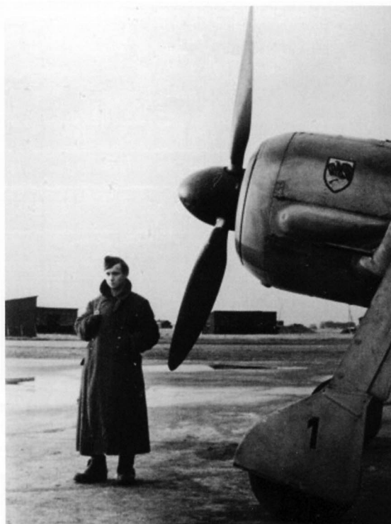
'Black 2' from 11./JG 5, an A-3, flying escort for a Ju 88 in early 1944. Note the style of the Gruppe wave, the fuselage bomb rack (not adapted for carrying drop tanks, lacking the sway braces) and the yellow spinner (Coll. Urbanke).
