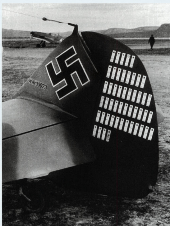
The tail section of 'Yellow 3' showing how the Werknummer had been masked off during the re-camouflaging process leaving a strip of RLM 79. The rest of the tail is in RLM 75 and RLM 70. There were 50 white victory bars on the rudder at the time this photograph was taken (Coll. Horst Kube).
