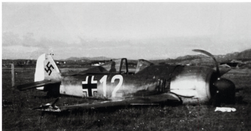
Fw 190A-2, W.Nr. 20287, 'White 12', of I./JG 5 after a landing mishap at Herdla on 14 July 1942 in which it suffered 40 per cent damage. Note the oversized numerals (without outline) and the factory finish of RLM 74/75/76 (Coll. Mombeek).
