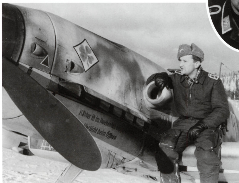
This series of photographs depicts the first Bf 109G-2/R-6 of Lt. Hans Döbrich in the winter of 1943. The light application of large splotches of white distemper on top of the normal grey camouflage can be seen to advantage, as well as the II. Gruppe emblem (a previous Staffel emblem and Döbrich's personal insignia) (Coll. Urbanke and Döbrich).
