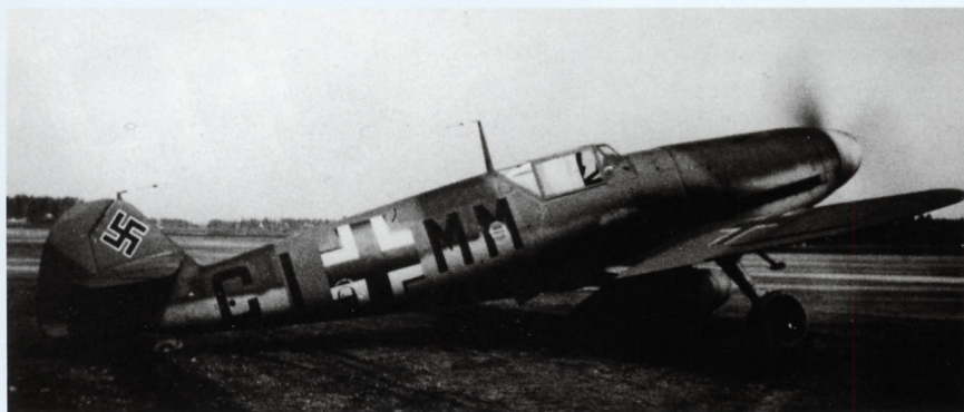
Bf 109F-4/trop, 'C1+MM', W.Nr 10173, at Pori on April 23rd 1943 en route to JG 5. It was probably not delivered to JG 5 before May as no Bf 109Fs are on record with II. Gruppe in April. Interesting points are over painted tail band and the drop tank. Also note heavy exhaust staining and recently applied service stencilling on fuselage (Via Hannu Valtonen).
