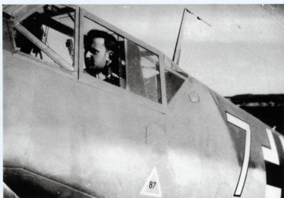
Hans Döbrich in the cockpit of a recently delivered Bf 109F-4/Trop, 'Yellow 7' of 6./JG 5. This shows to advantage the solid application of the two upper surface colours going half-way down the fuselage. It is significant to see that the canopy frames completely finished in the lightest upper surface colour, which suggests this is the original colour, whereas the darker colour seem to be recently applied as the finish is somewhat uneven (Coll. Döbrich).
