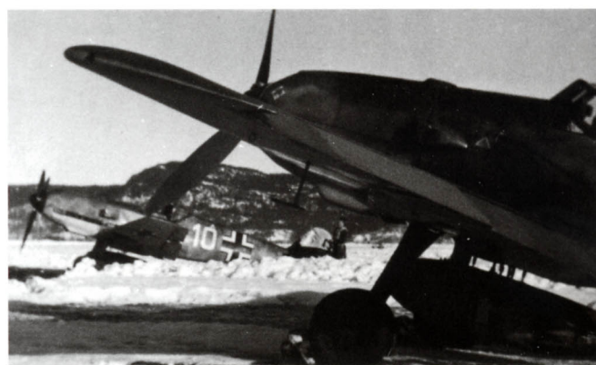
'White 12' of Einsatzstaffel/Jagdgr. Drontheim at Værnes during May/June 1942. The clover emblem of 6./JG 5 on the nose is noteworthy. Camouflage is the regular RLM 74/75/76 with evidence of considerable repainting. The undercarriage legs and insides of the undercarriage doors are RLM 66. Despite appearances, the ventral engine cowling is not yellow (compare with undercarriage door). The lower photo shows 'White 12' at an earlier date before the JFS insignia was applied, in company with 'White 10', probably the machine of Fw. Dombacher. A 300-litre drop tank is fitted (Coll. Brekken).
