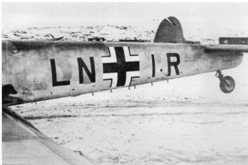
The fuselage of Bf 110 C-2, W.Nr. 3026, 'LN+IR' after coming to grief at Kirkenes airfield on 12 October 1941. This view clearly shows the frame numbers and what is probably the over-painted Stammkennzeichen, presumably using RLM 02. This aircraft was produced some two years previously and had definitely been repainted at least once since then. The colours used were RLM 74/75/76 with substantial mottling in RLM 02 on the sides. A ventral yellow fuselage band may have been present, but it is difficult to ascertain in this view (Coll. Dybvig).
