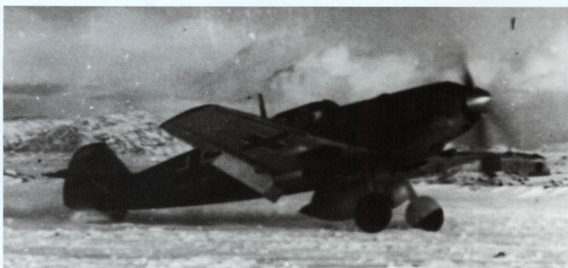
The highly polished spinner leaves no doubt as to the identity of this Emil taxiing on a snow-covered airfield during the winter of 1941-42. The flaps are deployed and the aircraft is fitted with a 300-litre drop tank, indicating that this was taken just before take-off, or alternatively, after landing, in which case the mission was an uneventful one (Coll. Brekken).
