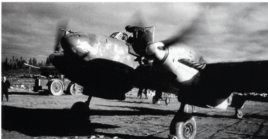
A Bf 110 E running up its engines. Note the extra air intake on the nose which was a distinguishing mark for the E-series and the external armoured wind shield. The spinners are not the usual type seen on the early series Bf 110s with an open type, but reminiscent of the capped spinner seen on the later Bf 109E-series (BA).
