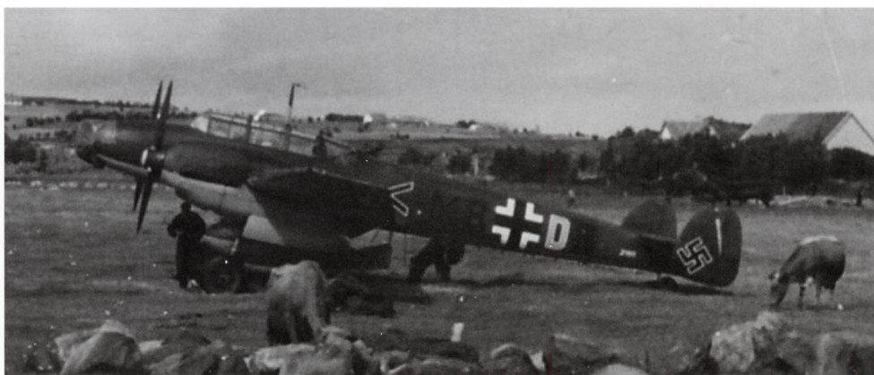
Another Bf 110 D-0 from Stab I./ZG 76, marked 'M8+DB' and with the single chevron of an adjutant. The camouflage is standard, but instead of the Dackelbauch, this Messerschmitt has been equipped with a ventral field-modified 900-litre drop tank installation (Coll. Dybvig).
