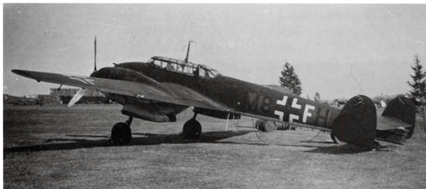
A Bf 110 D-0 of I./ZG 76 seen at Stavanger-Sola in early summer 1940. The aircraft is finished in the regular 70/71/65 scheme, but there is evidence of some over-painting around the fuselage codes, probably of the Stammkennzeichen. The extended tail section housing a dinghy shows this to be a D version, but note that a Dackelbauch is not fitted (Coll. Brekken).
