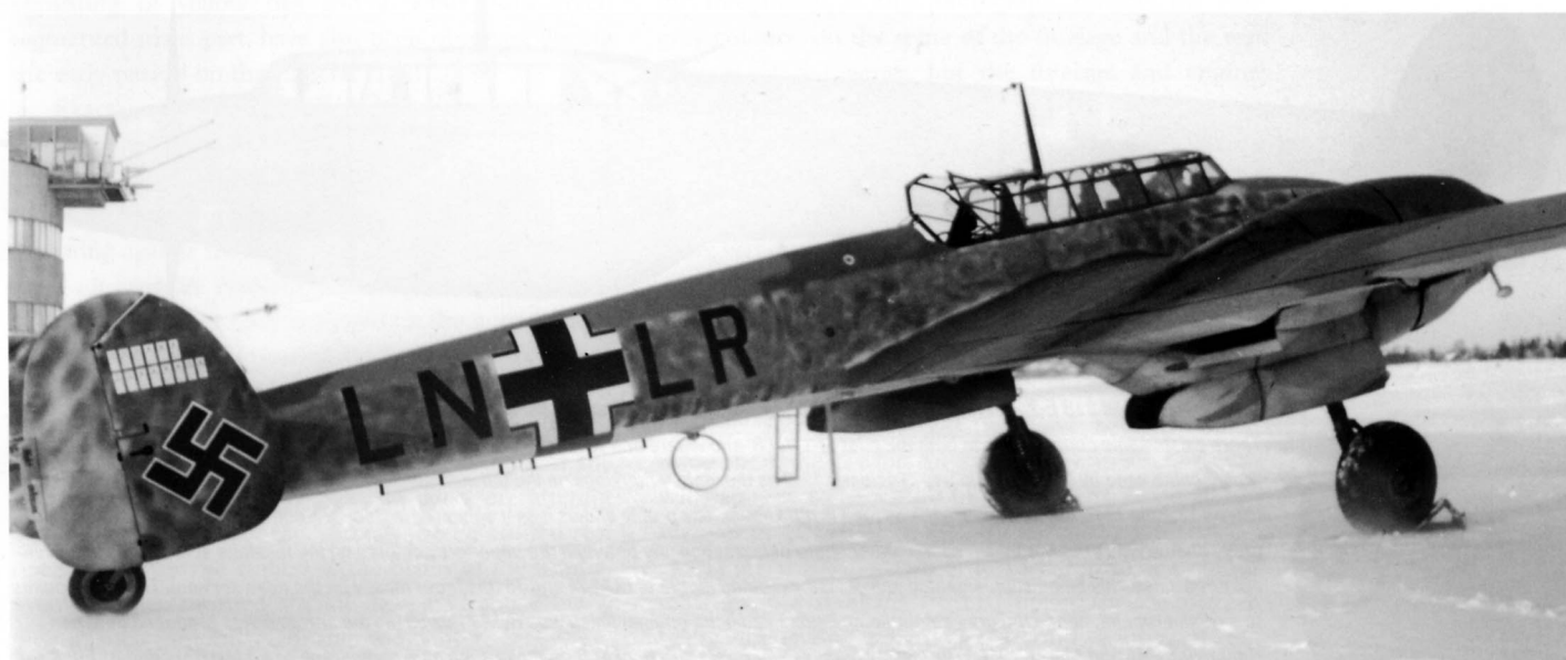
As the enlarged oil cooler and sand filter on the supercharger intake show, this is a Bf 110 E modified for tropical service. This is, in fact, the only tropical early series Bf 110 known to have served with JG 5, but unfortunately the code is not known. The sub-type can be determined by the air channel just discernible on the dorsal part of the MG cover lying on the ground beneath the aircraft. This was part of the new heating system introduced in the Bf 110 E series. The camouflage comprises the normal greys (BA).
