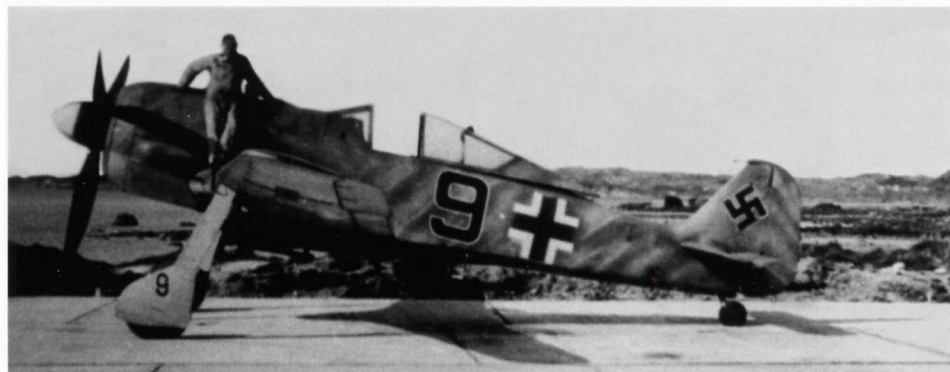
A quite unique Fw 190 from 2./JG 5 at Stavanger-Sola at the beginning of July 1942, just after the first aircraft of this type landed there. This indicates that the camouflage finish is fairly recent, consisting of streaks of RLM 74 and 75 over the basic grey factory scheme on fuselage sides and the rudder, these streaks being slightly accentuated on the fuselage by thin streaks of RLM 76. This special pattern was probably added locally, or in Denmark, just before hand-over to 2. Staffel. The individual number is again oversized and repeated in black on the undercarriage doors (Coll. Mombeek).
